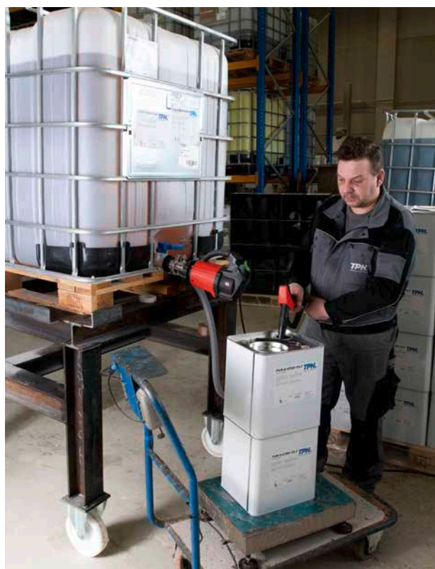
Fast container filling from the IBC outlet.
