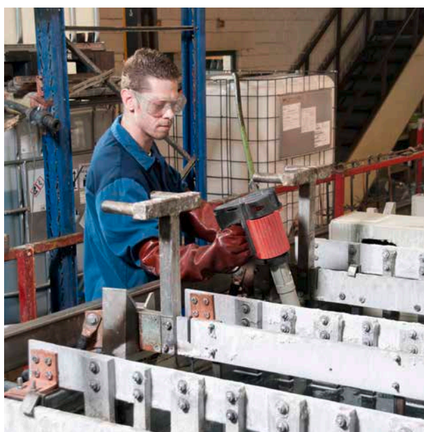
Emptying of an electroplated sink (F 424 PP).
