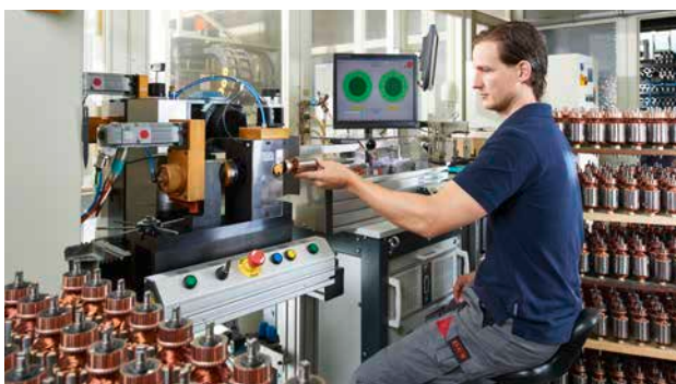
Anchor test in the winding department.
